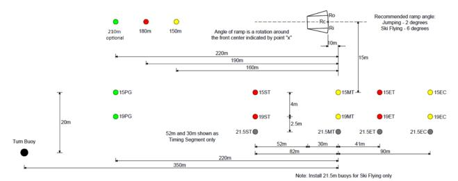
The ramp must be parallel to the jump course and slightly open. The tolerance for standard jumping is between  $+1.00^{\circ}$  and  $+2.50^{\circ}$  open.
